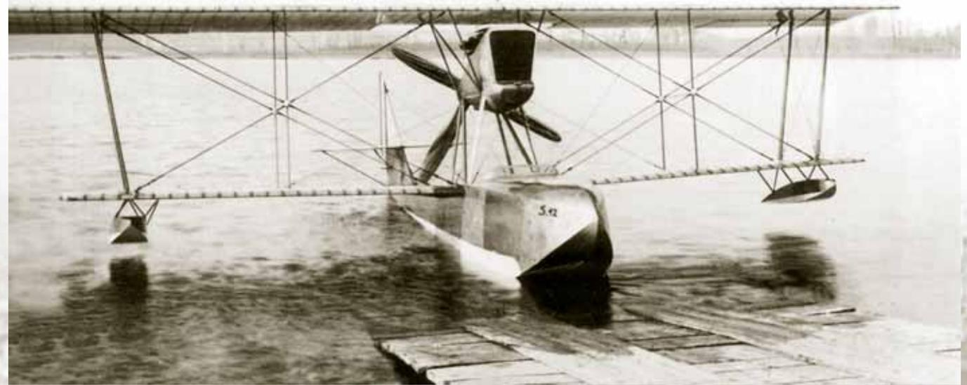
The SIAL Savoia S.2 fitted with an Ansaldo 550-hp motor was piloted by Luigi Bologna at an average speed of 107-mph to win the 1920 Venice event.
